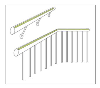
1 Handrail Markings Product Code: [H3-001] Description: [15.5mm wide aluminium (aluminum) base photoluminescent handrail strip suitable for curved handrails. Available in 1000mm and 3060mm lengths.]
