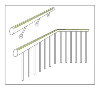
1 Handrail Markings Product Code: [H5-001] Description: [27mm wide aluminium (aluminum) base photoluminescent handrail strip suitable for curved handrails. Available in 1000mm and 3060mm lengths.]
