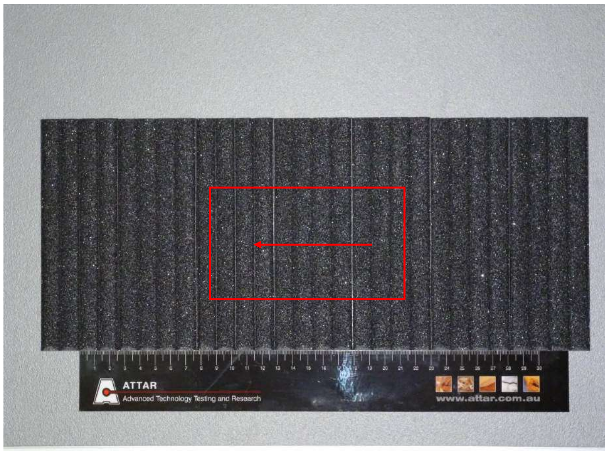
Figure 1: Ecoglo N3-070 contrast strip. Highlighted area and arrow indicates contact area and test direction.
