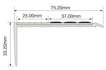
The F15-173 Step Nosing is designed to ensure visibility of steps in escape routes for compliance with NFPA Life Safety Code (NFPA 101) and International Fire Code (IFC), and any performance based building codes. The Step Nosing will be effective in all light conditions including during failure of the main lighting.
