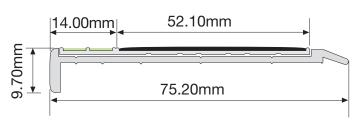
The F14-175 Step Nosing is designed to ensure visibility of steps in escape routes for compliance with International Fire Code (IFC), and any performance based building codes. The Step Nosing will be effective in all light conditions including during failure of the main lighting.
