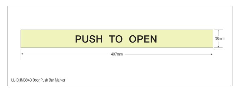
The UL-DHM3840 Door Push Bar Marker is designed to ensure visibility of panic bars on doors in escape routes for compliance with NFPA 101 Life Safety Code and International Fire Code (IFC). The Door Push Bar Marker will be effective in all light conditions including failure of the main lighting.
