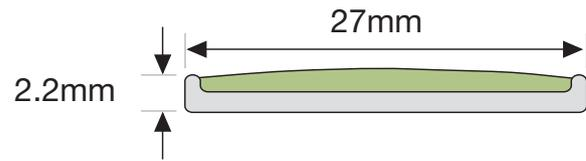
The MS-26 Handrail Wall Strip is designed to ensure visibility of specified building features in escape routes for compliance with performance based building codes. The Handrail Wall Strip will be effective in all light conditions including during failure of the main lighting.
