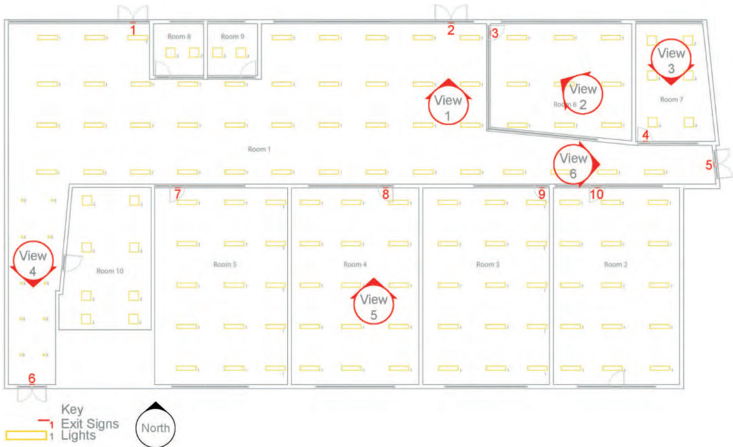
Room layout used for natural lighting model (electric lights turned off)
