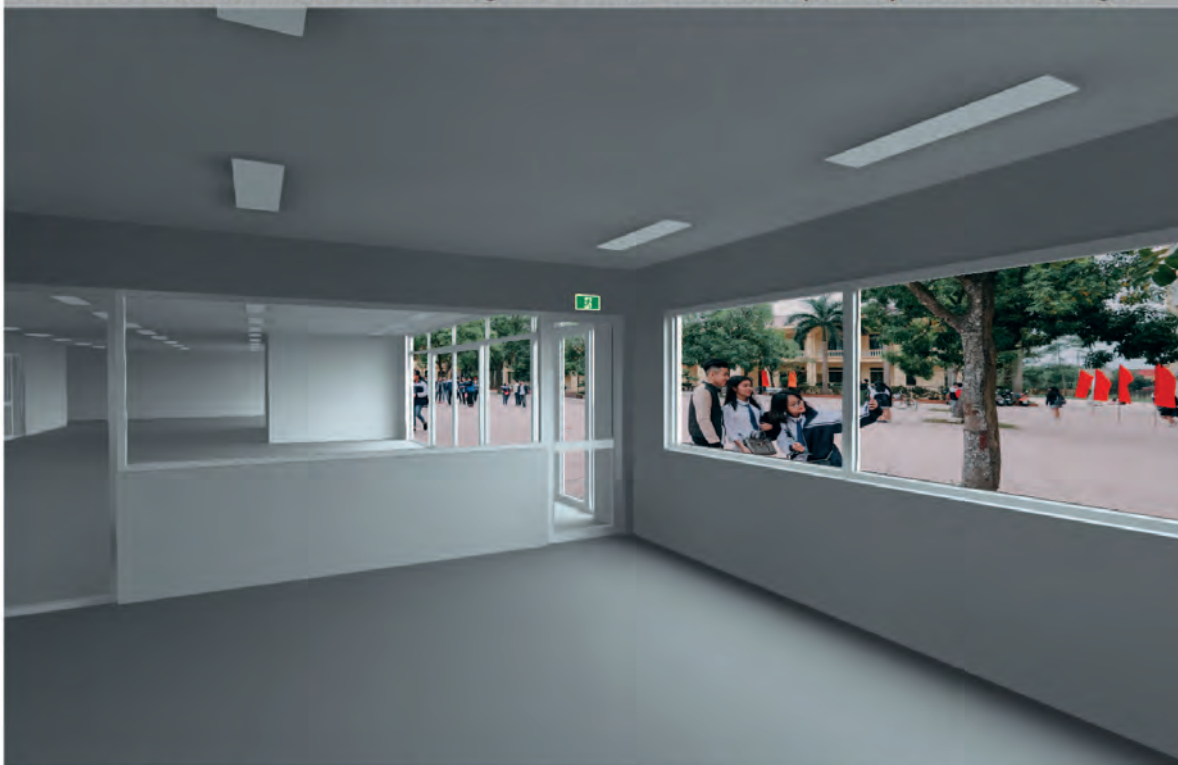
View 2. 40 lux illuminance on the sign for a min. of 6 hours per day from natural light.
