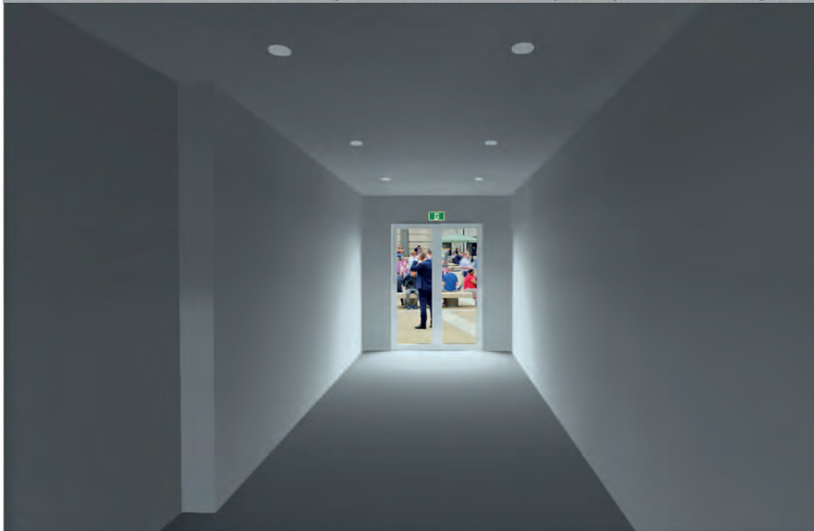
View 4. 30 lux illuminance on the sign for a min. of 6 hours per day from natural light.
