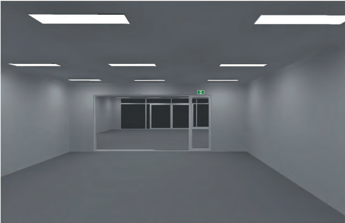
View 5. 258 lux illuminance on the sign from electric lighting.
