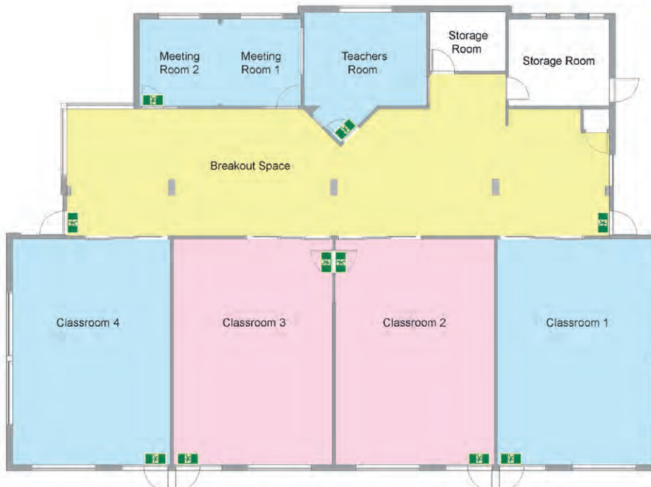
Fig. 5b. School Block where the escape routes are through adjacent classrooms that may not be occupied.
